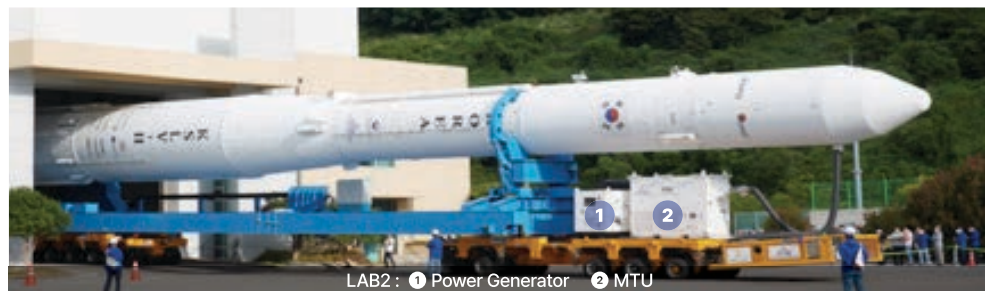
LAB2 : ① Power Generator ② MTU
