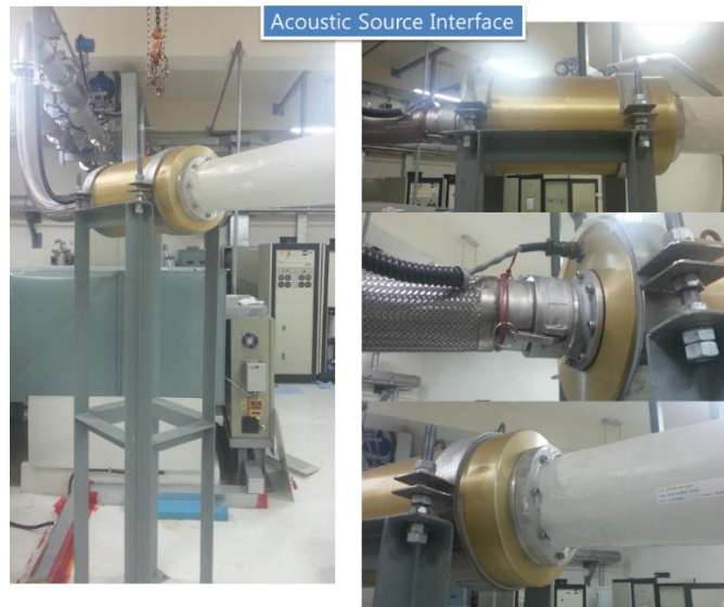
Figure 3 Acoustic horn and pipe interface
